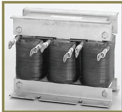
**A line reactor reduces discontinuity of the current drawn by a VFD's converter, which in turn reduces the harmonic current.**
