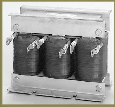
**A line reactor reduces discontinuity of the current drawn by a VFD's converter, which in turn reduces the harmonic current.**
