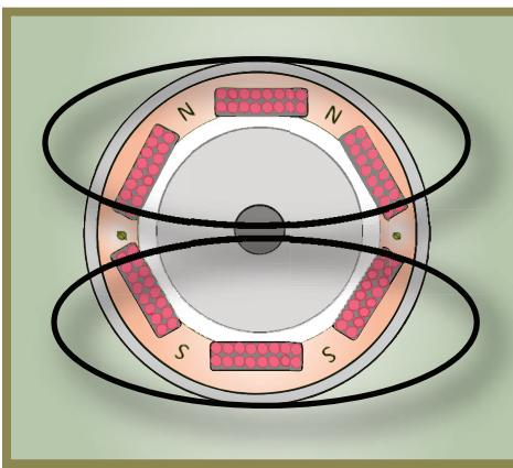
**The number of poles in a motor is one of the factors used to determine the motor's torque per hp and rpm per Hz.**
