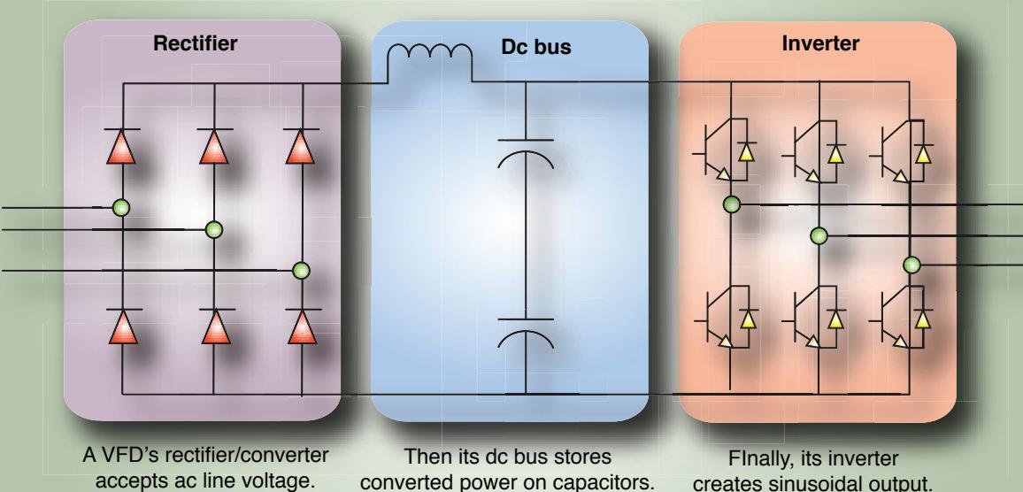
(IGBTs) connected in a full-wave bridge configuration.
