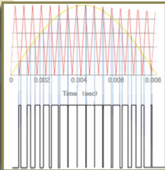
**Carrier frequency** is the rate at which output transistors are gated or turned on.
