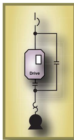
A two-contactor bypass is a VFD accessory that allows motor operation across the line or through the VFD. It can be used to run the motor at a constant speed directly from the incoming line in case of VFD failure.
