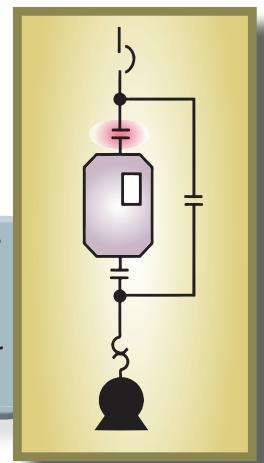
A three-contactor bypass allows a motor to be run directly from the incoming line, bypassing the VFD. This is useful during VFD servicing, and can be used to run the motor at constant speed at a higher efficiency than with the VFD in circuit.
