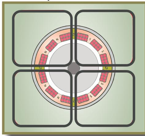
Coils are wrapped around symmetrical iron cores, in turn arranged around the stator's inner diameter.
