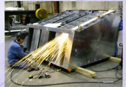
Transitioning NMR silencer for kitchen exhaust with removable casings for cleaning
