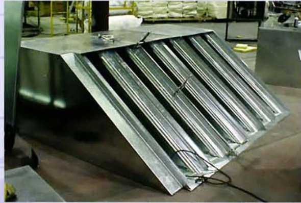
RPG with mitered inlet connection
