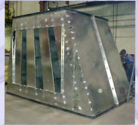
RMP transition with bypass opening
