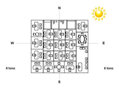
As the occupant loads change throughout the day, a VRF heat recovery system can shift the capacity to meet the load.
