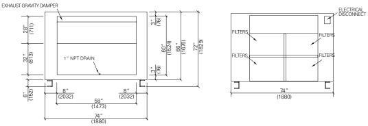
\* If optional Heat and Cooling is not selected, deduct 30" from overall length. A service clearance equal to the width of the unit is required on both sides.
