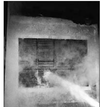
UL 555 Hose Stream Test
