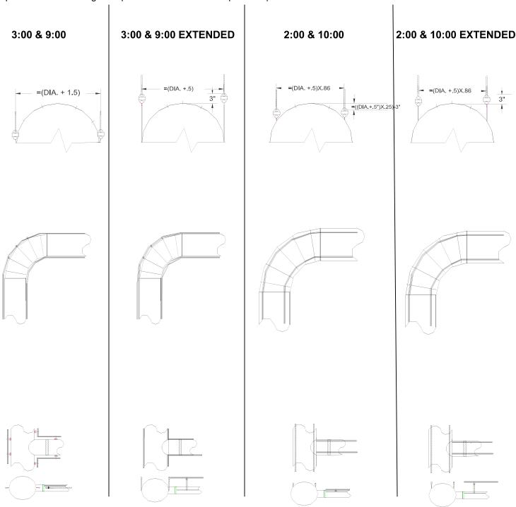
Note: The previous drawings illustrate possible double rail suspension systems. Since every installation is different, support brackets are not supplied. Triple suspension systems used on larger diameters systems
