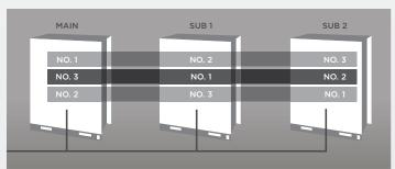
Systems with multiple condensing units will cycle the lead condensing unit operation upon startup to extend system life. In the event that a fault is detected in the master unit, one of the other condensing units can be configured as the master unit, allowing the system to continue operation.
