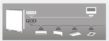
For easier installation and setup, communication wiring can be shared by multiple indoor and outdoor units.
