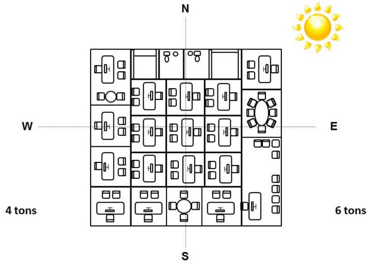
As the occupant loads change throughout the day, a VRF heat recovery system can shift the capacity to meet the load.
