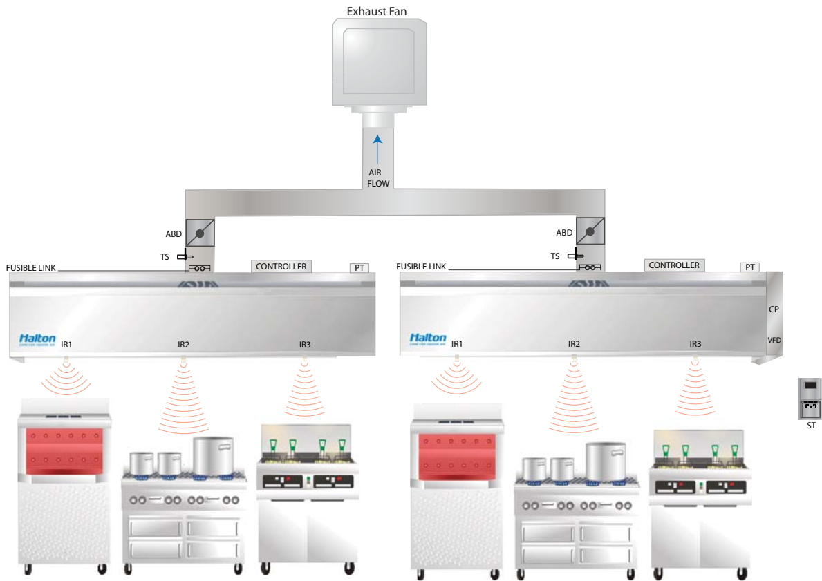
Figure 2: Multiple Hood M.A.R.V.E.L. Installation
