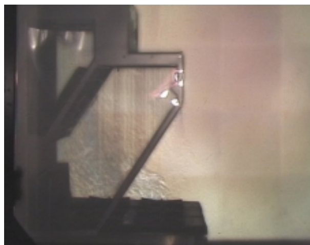
Photo 4 Schlieren Image of KVL Hood. Capture Jet™ On
