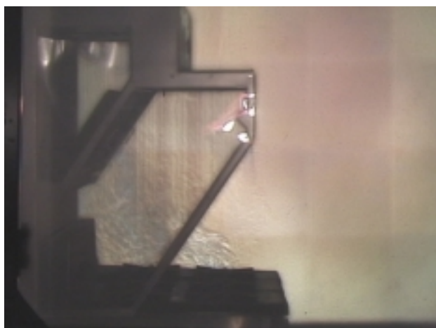
Photo 2 Schlieren Image of KVE Hood. Capture Jet™ On
