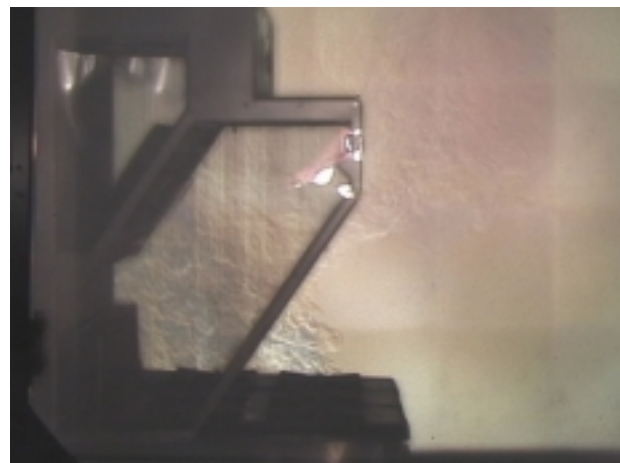
Photo 1 Schlieren Image of KVE Hood. Capture Jet™ Off
