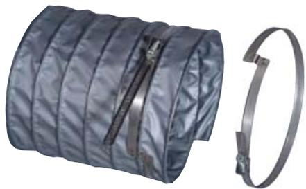
Bridging over helix allows for better contact of clamp to duct thus lowering leakage
